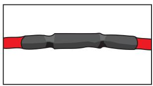
Wait for the butt splice to cool, slip heatshrink over the joint and heat.
