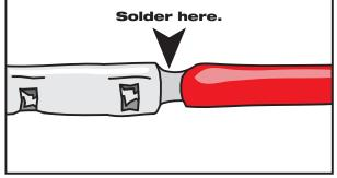
Solder the wires to the butt splice. Ensure that a good connection is made.
