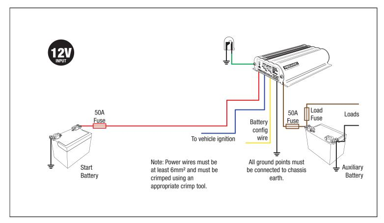
Figure 2.3 - Standard setup for a 12V Start Battery
