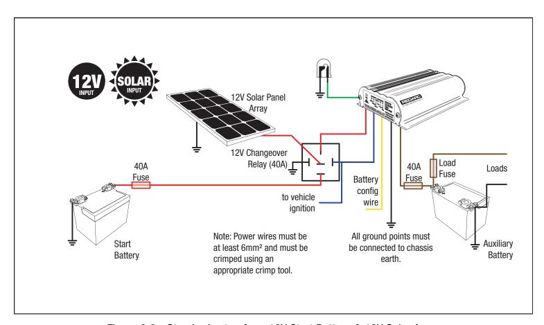
Figure 2.2 - Standard setup for a 12V Start Battery & 12V Solar Array
