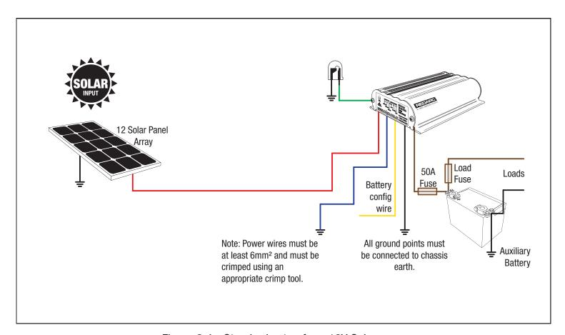
Figure 2.4 - Standard setup for a 12V Solar array
